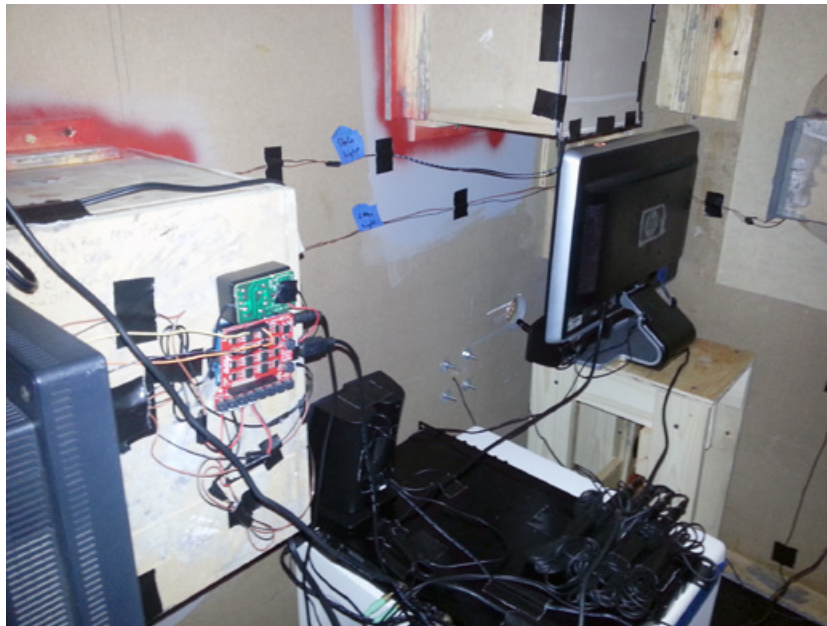
Figure 6. Main circuit inside the structure consisting of microcontrollers, displays, a firewire interface, and an Apple-Mini
